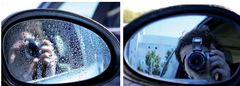
Fig. 43. Automotive mirror, left: uncoated, right: coated with \text{TiO}_2 . (Reproduced from Energy Environ. Sci. 5 (2012) 7491–7507 with permission from Royal Society of Chemistry).
